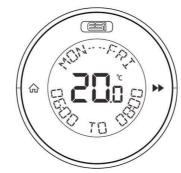
The display will show the start time (flashing), and end time for Program 1, e.g. 06:00 TO 08:00 Use the DIAL to adjust the start time & press ▶ to move to the end time. The end time will flash, use the DIAL to adjust the end time & press ▶ to move on to the temperature. Use the DIAL to adjust the temperature & press ▶ to confirm your settings for Program 1.
