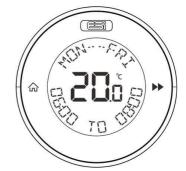
The display will show the start time (flashing), and end time for Program 1, e.g. 06:00 TO 08:00 Use the DIAL to adjust the start time & press ▶ to move to the end time. The end time will flash, use the DIAL to adjust the end time & press ▶ to move on to the next program
