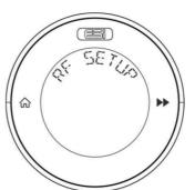
On your ESWIFIHUB, hold the right button (Wi-Fi) until the left button (RF) flashes green. On your ESi CIRRUS, hold the ▶ button until the display shows RF SETUP Tap ▶, the display will show RF PAIR PAIRING with a number counting upwards. When your ESi CIRRUS & ESWIFIHUB are paired, you will see SAVING at the bottom of the screen.
