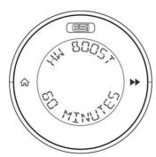
Hold the HOME button until HW BOOST is displayed at the top of the screen & 60 MINUTES shows at the bottom of the screen.
