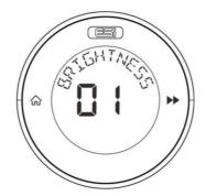
Use the DIAL to adjust the screen brightness (1 to 10) Press > to save your setting and tap the HOME button to exit the menu.
