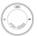
The bottom of the display will show PIN 0000. . Use the DIAL to scroll through the digits & ▶ ▶ to move to the next digit When you have entered your PIN, Tap ▶ ▶
