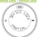
Tap ▶ ▶ and use the **DIAL** to navigate to DEVICE LOCK. Tap ▶ ▶. You will see PARTIAL at the bottom of the screen.
