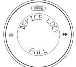
Tap ▶ ▶ and use the **DIAL** to navigate to DEVICE LOCK. Tap ▶ ▶ & you will see FULL at the bottom of the screen.
