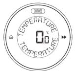
Press ▶ ▶, the display will show TEMPERATURE CALIBRATION at the top of the screen and 0.0°C flashing in the centre of the screen.
