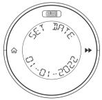
The display will show SET DATE at the top of the screen & a date at the bottom of the screen.
