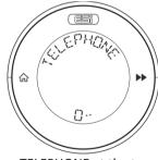
The display will show TELEPHONE at the top of the display and -- at the bottom of the display. Use the **DIAL** to scroll through the numbers and use ▶ ▶ to move to the next number. When you have finished, tap ▶ ▶ to save your setting. Tap the **HOME** button until you get back to your home screen.
