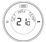
SET MAX TEMPERATURE will show at the top of the screen screen & a temperature in the centre of the screen e.g. 21.0°C.
