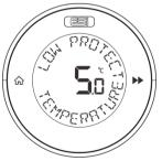
Press ► ►, the display will show LOW PROTECT TEMPERATURE and 5.0°C in the centre of the screen. Use the **DIAL** to select a temperature which you would like as a frost protection temperature setting (between 0.5°C and 20.0°C)
