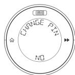
The screen will show CHANGE PIN at the top, and NO at the bottom of the screen. Use the **DLAT** to select YES or NO
