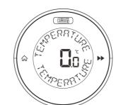
Press ▶ ▶, the display will show TEMPERATURE CALIBRATION at the top of the screen and 0.0°C flashing in the centre of the screen.
