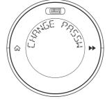
The display will show CHANGE PASSWORD. If you don't want to change the PIN, use the **DIAL** to enter the Landlord Settings and move onto the next step below. To change the PIN, tap ▶ ▶ and use the **DIAL** to scroll through the numbers and use ▶ ▶ to move to the next number. When you have entered a new PIN press ▶ ▶
