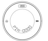
The bottom of the display will show PIN 0000. Use the **DIAL** to scroll through the digits and ▶ ▶ to move to the next digit. When you have entered your PIN, Tap ▶ ▶
