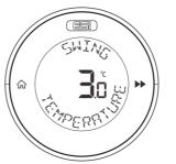
Use the **DIAL** to adjust the **SWING** setting (0.1°C to 3.0°C).
