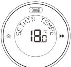
SET MIN TEMPERATURE will show at the top of the display & a temperature in the centre of the display e.g. 18.0°C.
