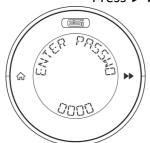
The display will show ENTER PASSWORD (PIN) at the top of the screen and 0000 at the bottom of the screen. Use the **DIAL** to scroll through the numbers and use ▶ ▶ to move to the next number. The default PIN is 0000. When you have entered the PIN, tap ▶ ▶
