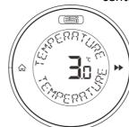
Use the DIAL to adjust the number in the centre of the screen  $(-3.0^{\circ}\text{C to } +3.0^{\circ}\text{C})$ .
