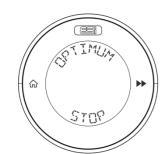
Turn the **DIAL** clockwise to see OPTIMUM STOP. Press ▶ ▶ to enter Optimum Stop menu Use the **DIAL** to choose between ON & OFF.
