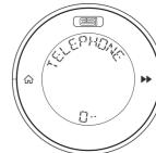
The display will show TELEPHONE at the top of the display and - - at the bottom of the display. Use the **DIAL** to scroll through the numbers and use ▶ ▶ to move to the next number.
