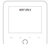
Use **AV** to choose between HEATING & **HOT WATER or HEAT** ONLY. Press **HOME** to save. Use the **RETURN BUTTON** to
