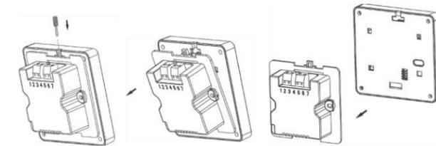
2. Fix the 35mm back box, terminals at the top, onto a 2 flange metal back box with 2 BM3.5x23 screws. If installing on a 4 flange metal back box, simply push down the flanges on the top and bottom to leave the flanges on the left and right hand side.
