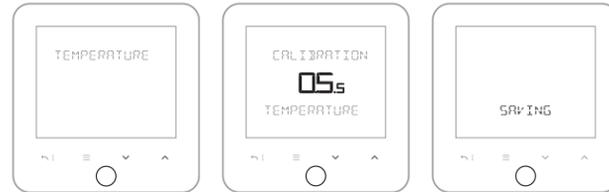
USE the to navigate to the TEMPERATURE CALIBRATION menu and touch the home button to enter menu.
