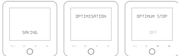
Touch the home button to enter optimisation settings. Navigate to OPTIMUM STOP by using .
