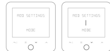
To choose the desired AOD setback navigate to MODE settings by using then press the home button to enter settings.
