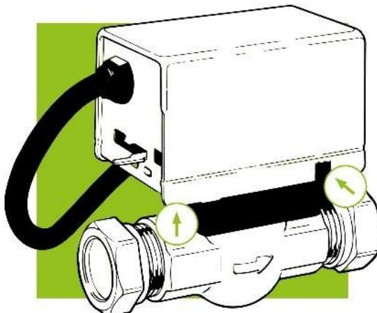
Firmly pull the actuator head away from the valve body. Failure to hold the release button can cause the retaining clip holding the valve body to the actuator to snap.
