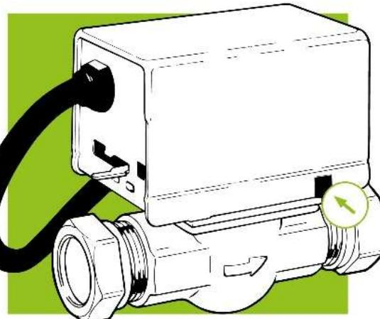
Press & hold the release button on the side of the actuator.
